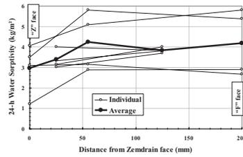
Figure 5. Water sorptivity variation with distance from “Z” face.
