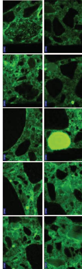
Figure 6. Microstructure of “F” (l.) and “Z” (r.) faces with depth from top to bottom. Each frame covers ≈ 5 mm depth.
