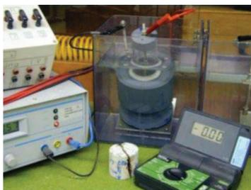
Figure 3. Chloride migration test on Ø50 × 50 mm core.
